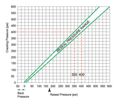
Example: For a valve set to crack at 400 psi, the minimum reseal pressure would be 350psi.
